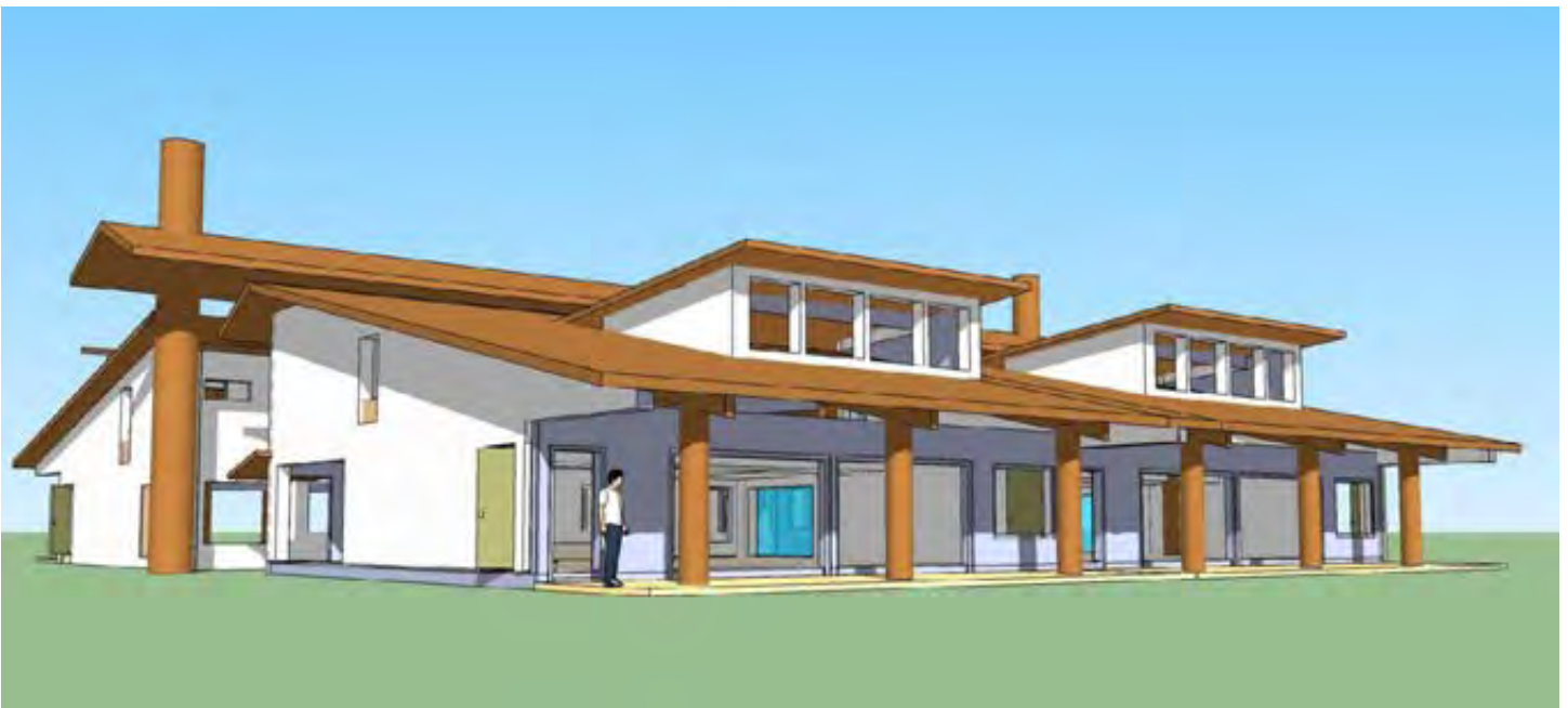
Covering the breezeway for weather protection
